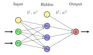
Figure 4.5: A Single-Layer Feedforward Neural Network with Biases shown explicitly
